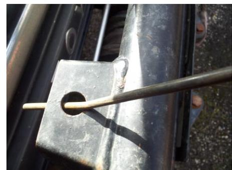
Its also worth running a 5mm drill bit up the holes in the base that the sticks push into as often swarf get left in and the sticks don't seat fully home. Usually ends in a loud twang as the stick jumps out as the wind gets up and then a clang as it falls onto your car. Followed by 6 hours of loud flapping .....
